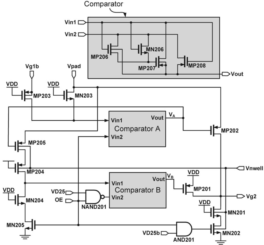
Fig. 11. Dual-path gate-tracking circuit.
