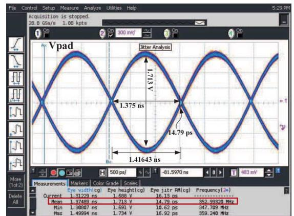
Fig. 14. The eye diagram of  $V_{\text{pad}}$  with VDDIO = 2.5 V in Tx mode.
