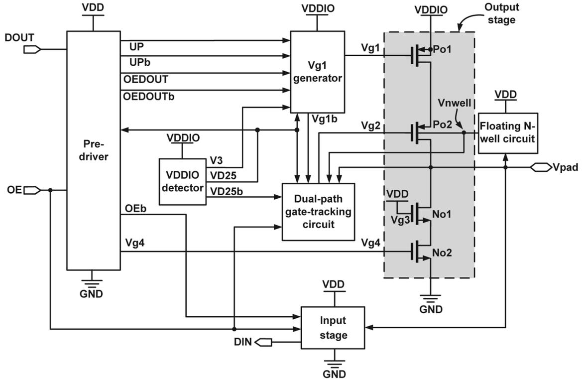
Fig. 4. The proposed mixed-voltage I/O buffer.
