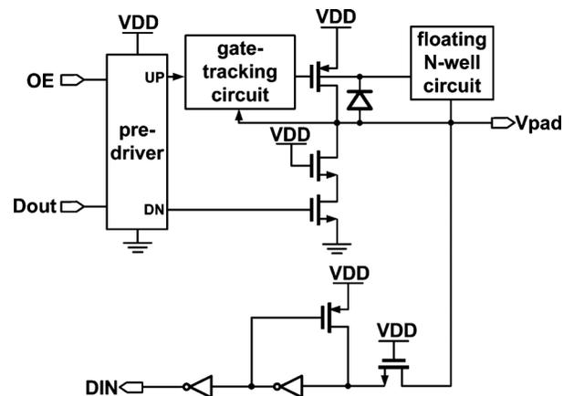
Fig. 1. Type I mixed-voltage I/O buffer with the gate-tracking and floating N-well circuits.
