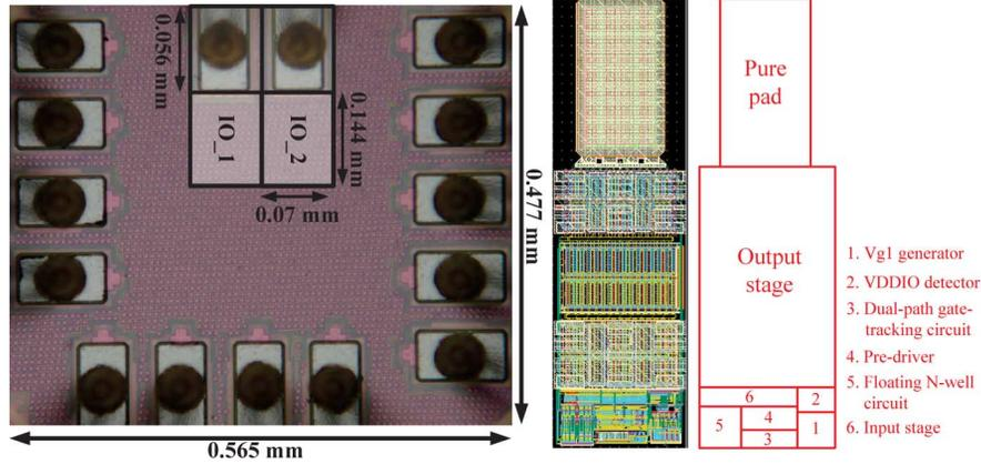
Fig. 12. Die photo of the proposed mixed-voltage I/O buffer.
