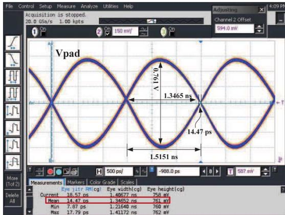
Fig. 15. The eyes diagram of the proposed design in Rx mode.
