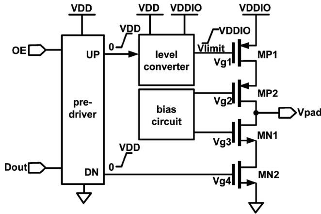
Fig. 2. Type II mixed-voltage I/O buffer with the level converter and bias circuit.
