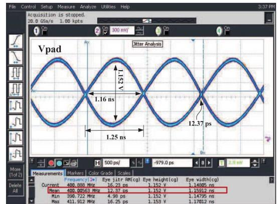
Fig. 13. The eye diagram of  $V_{\text{pad}}$  with VDDIO = 1.2 V in Tx mode.
