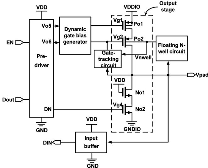
Fig. 3. Type III mixed-voltage I/O buffer with the gate-tracking circuit, floating N-well circuit and dynamic gate bias generator.
