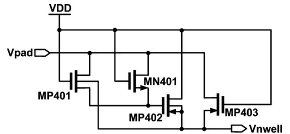
Fig. 8. Floating N-well circuit.
