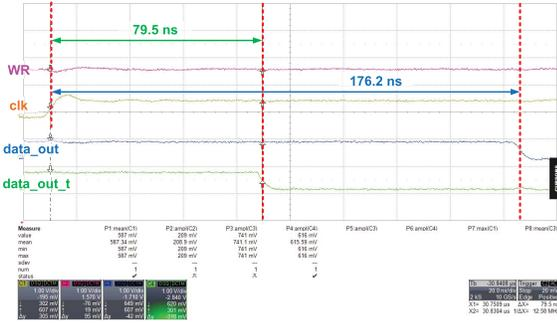
Fig. 20. Demonstration of the measured read delay compensation at 0.6 V system voltage.
