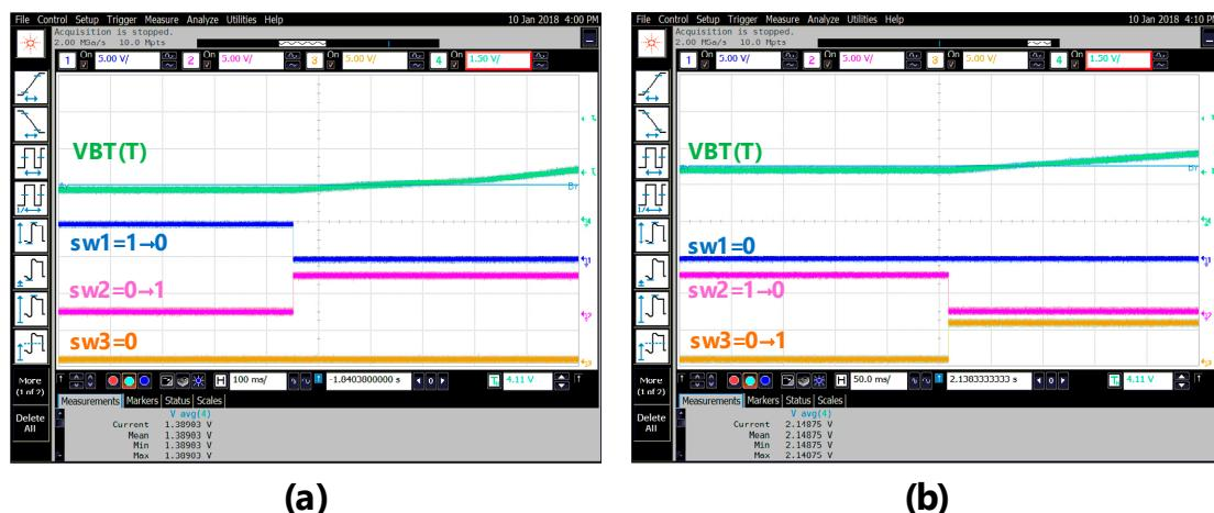
**Figure 11.** The scenario of three switches when the ambient temperature (a) 70–65  $^{\circ}\text{C}$  and (b) 30–25  $^{\circ}\text{C}$ .
