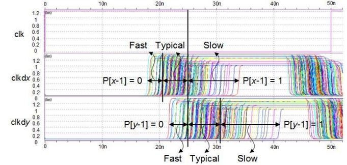
Fig. 11. Postlayout simulation of PVT detector.
