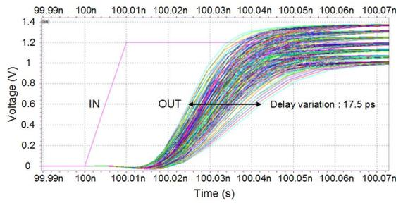
Fig. 9. Delay variation without PVT detection.
