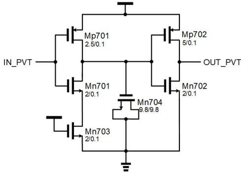
Fig. 5. Delay cell in PVT detector (W/L in  $\mu\text{m}$ ).
