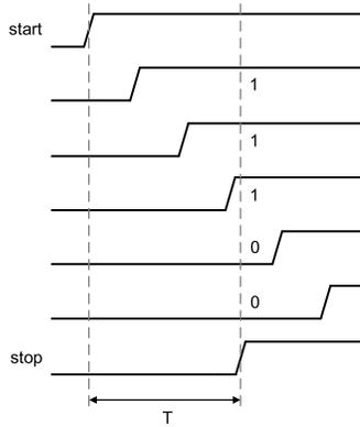
Fig. 3. Timing diagram example of our TDC.
