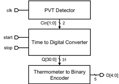
Fig. 1. Block diagram of the proposed TDC.
