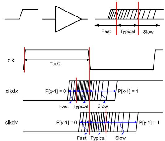
Fig. 6. Classification by stages 24 and 29 of the PVT detector.
