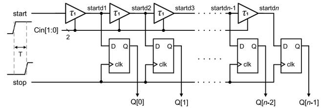
Fig. 2. Schematic of TDC in Fig. 1.
