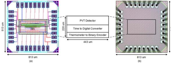
Fig. 8. (a) Layout of the proposed TDC. (b) Die photograph.
