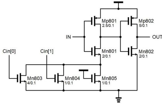
Fig. 7. Delay cell in TDC core (W/L in  $\mu\text{m}$ ).
