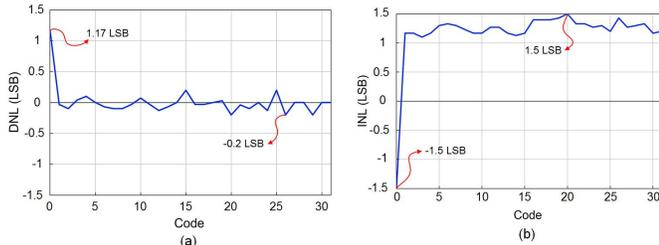
Fig. 14. Measurement of (a) DNL and (b) INL.
