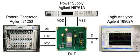
Fig. 12. Measurement setup.
