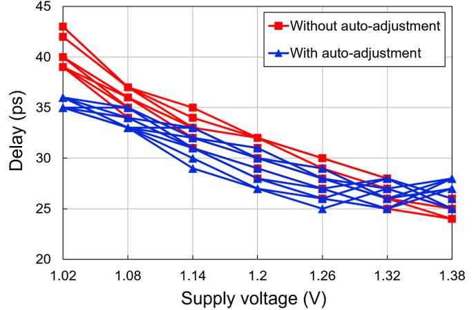
Fig. 17. Delay variation comparison given different VDD by measurement.
