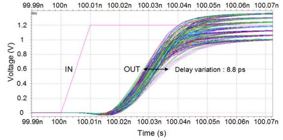
Fig. 10. Delay variation with PVT detection.
