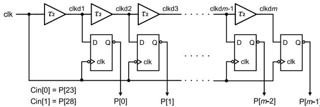
Fig. 4. Schematic of PVT detector.
