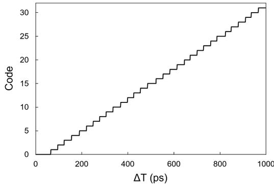
Fig. 13. Transfer function of the proposed TDC.
