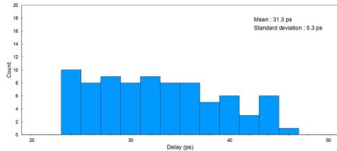
Fig. 15. Delay distribution without PVT detection by measurement.
