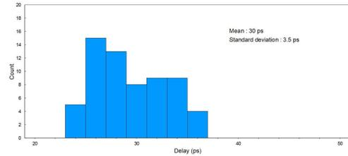
Fig. 16. Delay distribution with PVT detection by measurement.
