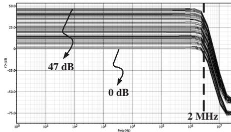
Fig. 12. Simulated waveform of the gain of the baseband circuit from 0 dB to 47 dB.
