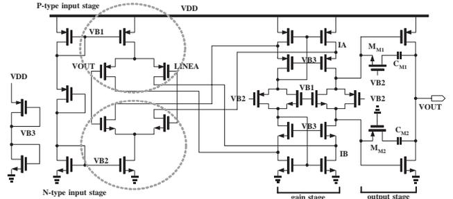
Fig. 9. Schematic of the rail-to-rail OTA.
