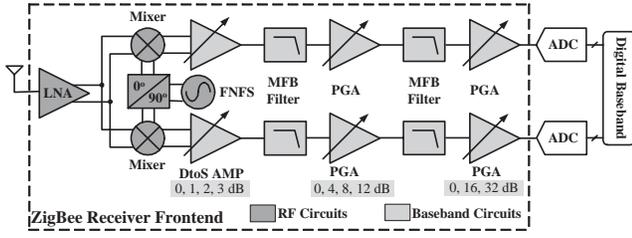
Fig. 2. Block diagram of the proposed ZigBee receiver.
