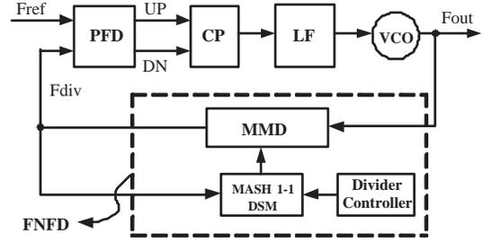
Fig. 4. Block diagram of the fractional-N frequency synthesizer.
