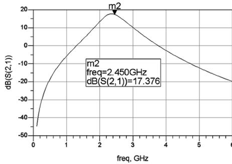
Fig. 11. Simulated waveform of the gain of the LNA at 2.45 GHz for the worst-case of SS, 70°C.
