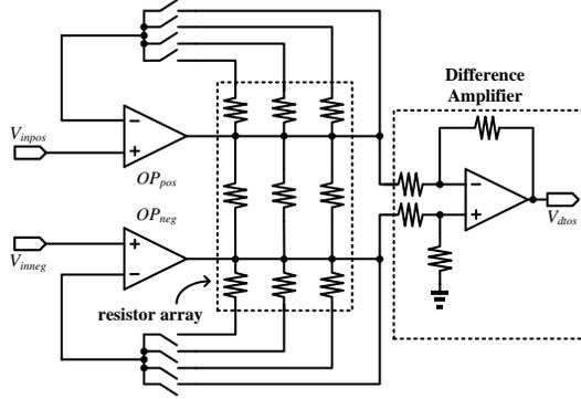
Fig. 7. Schematic of the differential-to-single-ended amplifier (DtoS AMP).
