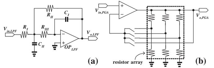
Fig. 8. Schematic of (a) the MFB filter and (b) the PGA.
