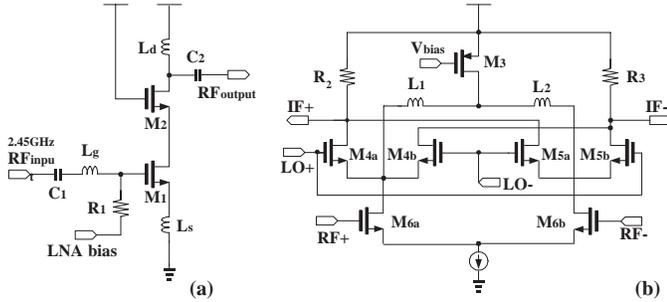
Fig. 3. Schematic of (a) the LNA and (b) the Mixer.
