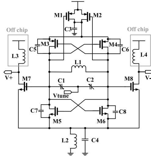
Fig. 5. Schematic of the VCO.
