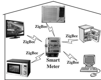
Fig. 1. The applications of ZigBee utilized in the HAN with the smart meter.
