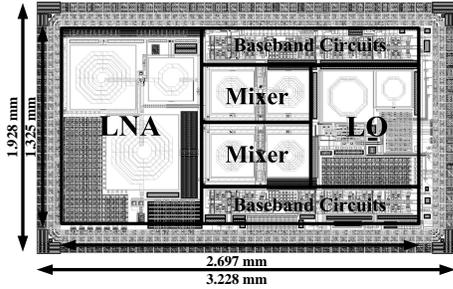
Fig. 10. Layout of the proposed ZigBee receiver.
