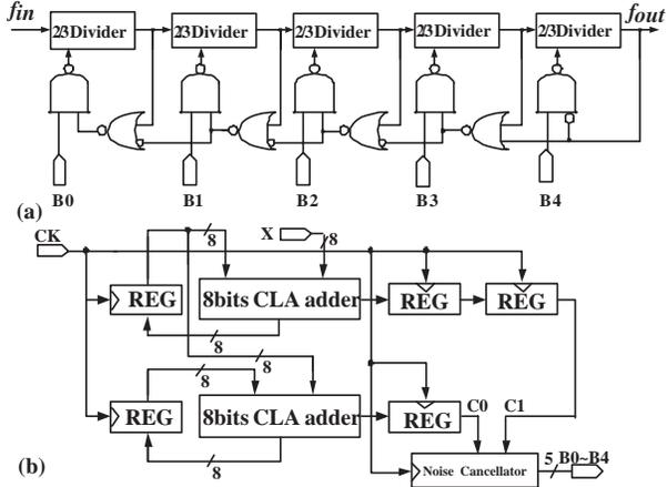
Fig. 6. Block diagram of (a) the multi-modulus divider (MMD) and (b) the MASH 1-1 DSM.
