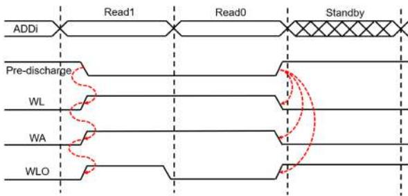
Fig. 5. Read cycle timing
