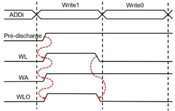
Fig. 6. Write cycle timing
