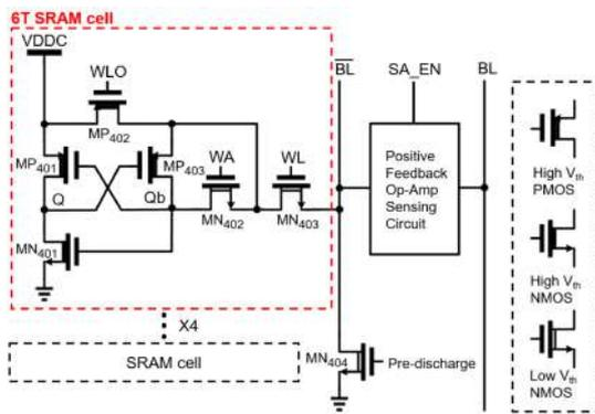
Fig. 2. Proposed 6T SRAM cell to enlarge SNM
