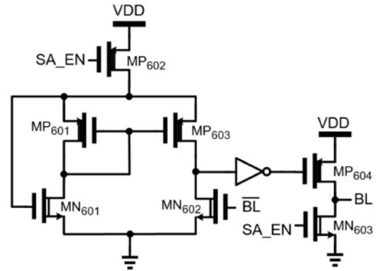
Fig. 3. Positive feedback op-amp sensing circuit
