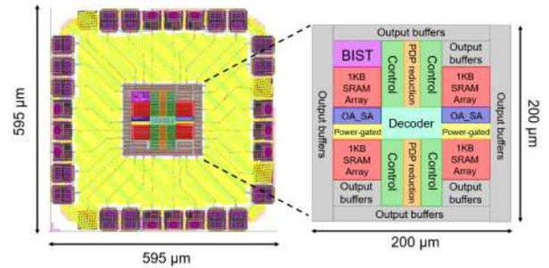
Fig. 7. Layout of the proposed 1-kb SRAM
