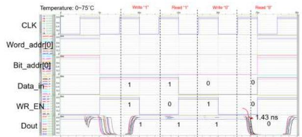
Fig. 8. All-PVT-corner post-layout simulation
