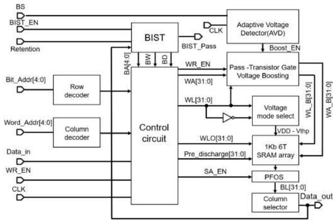
Fig. 1. Proposed low energy-consuming SRAM system diagram
