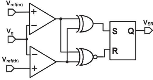
Fig. 3. 2-level Miller plateau detector circuit
