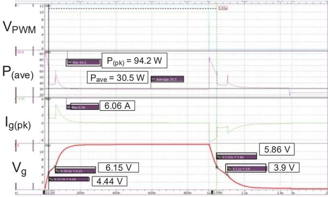
Fig. 7. TT,  $V_{DD} = 12\text{V}$ ,  $25^\circ\text{C}$  post-layout simulation
