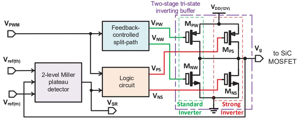
Fig. 1. Proposed SiC MOSFET AGD block diagram
