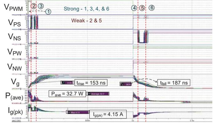
Fig. 6. All-PVT corners post-layout simulation of the proposed design
