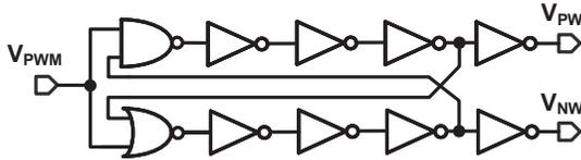
Fig. 4. Feedback-controlled split-path schematic [10]
