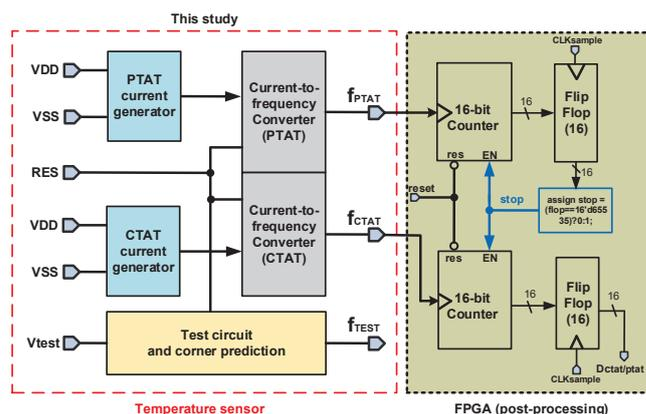
Fig. 1. Temperature detector architecture
