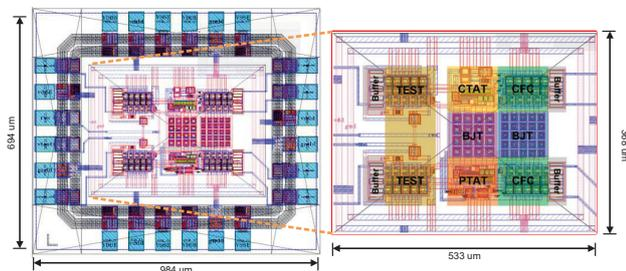
Fig. 6. Layout of the temperature detector
