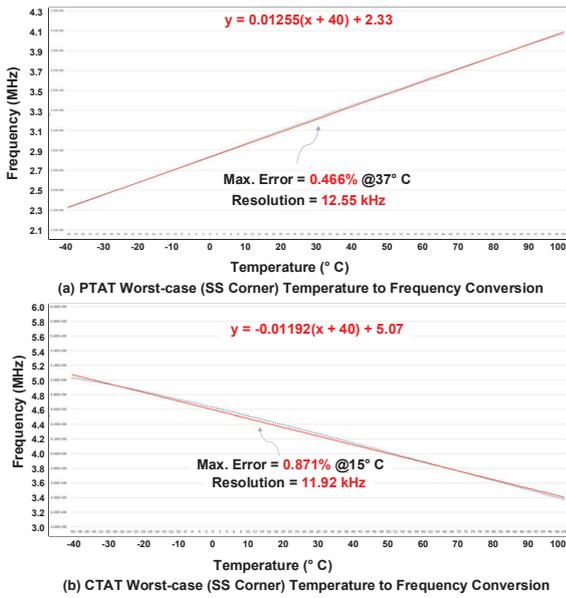
Fig. 8. Temperature vs. frequency simulation, (a) PTAT worst-case (SS); (b) CTAT worst-case (SS)
