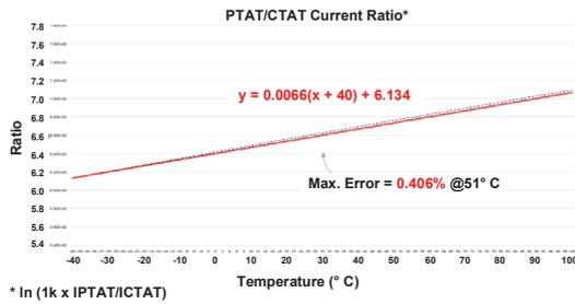
Fig. 9. PTAT/CTAT current ratio vs. frequency.  $f = \ln(1000 \times \frac{I_{PTAT}}{I_{CTAT}})$
