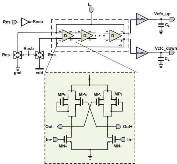
Fig. 4. Current-to-frequency converter
