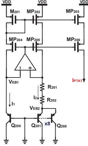
Fig. 2. PTAT current generator circuit
