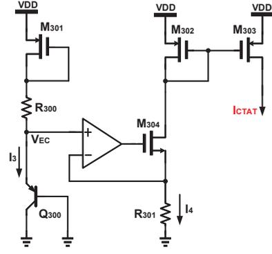
Fig. 3. CTAT current generator circuit
