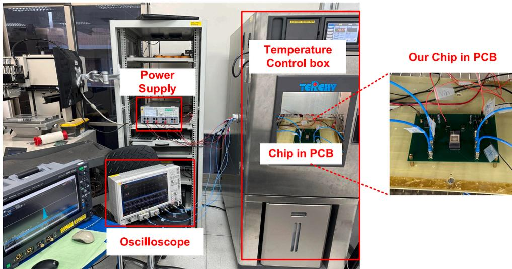
Fig. 5. Measurement setup at TSRI, Tainan.
