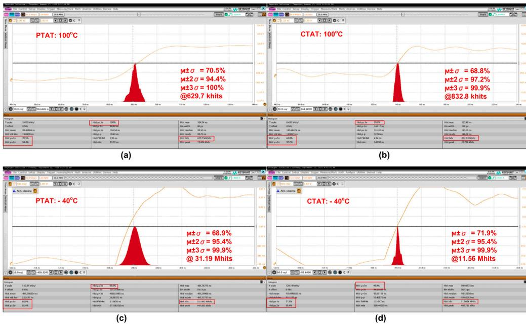
Fig. 12. Histograms of (a) PTAT at 100 °C; (b) CTAT at 100 °C; (c)PTAT at -40 °C and; (d) CTAT at -40 °C.
