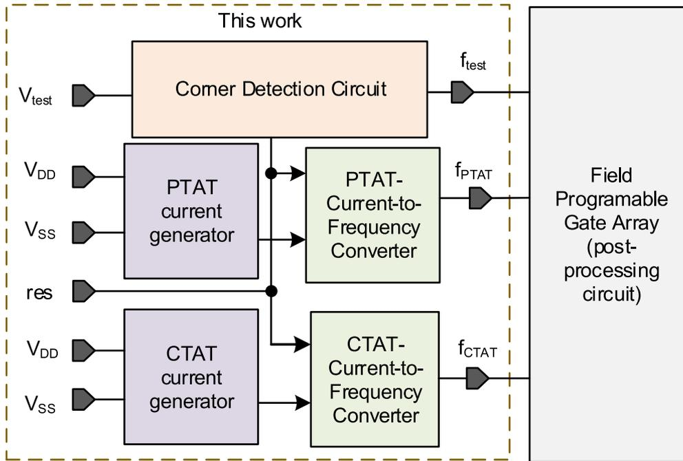
Fig. 1. Temperature sensor architecture.
