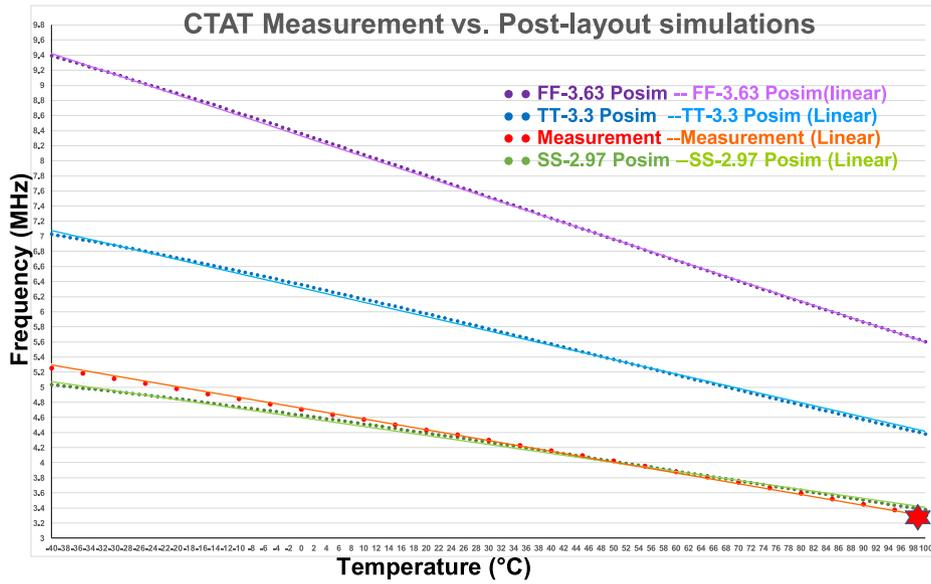
Fig. 8. The CTAT temperature vs. frequency curves for TT, FF, SS corners.
