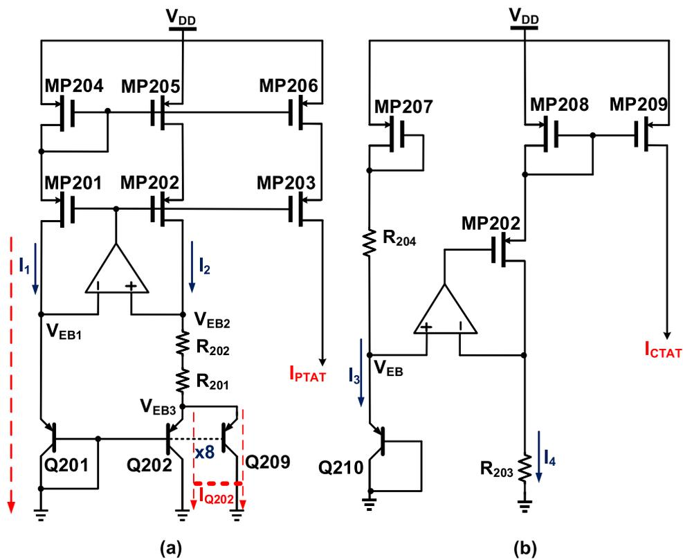
Fig. 2. (a) PTAT current generator; (b) CTAT current generator.
