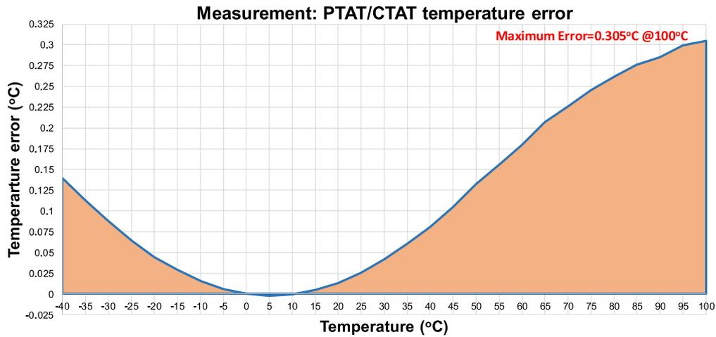
Fig. 11. Measured temperature error.
