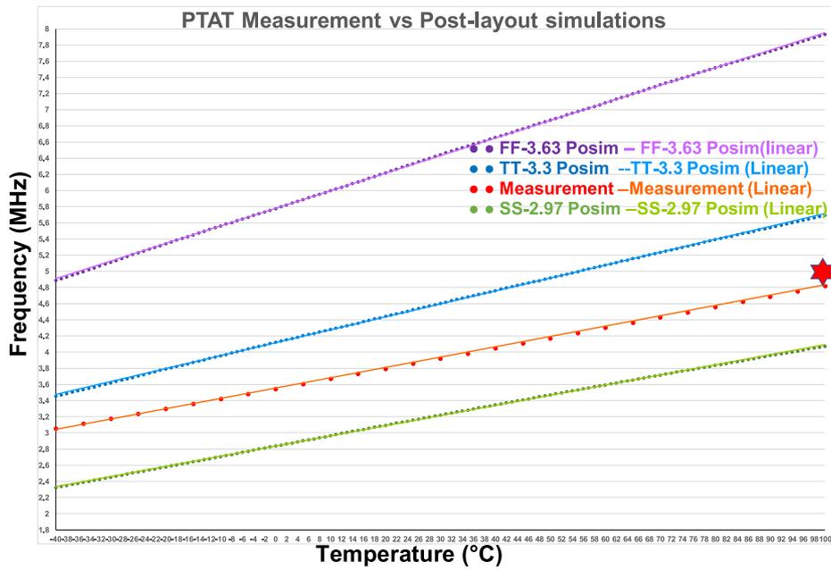
Fig. 7. The PTAT temperature vs. frequency curves for TT, FF, SS corners.
