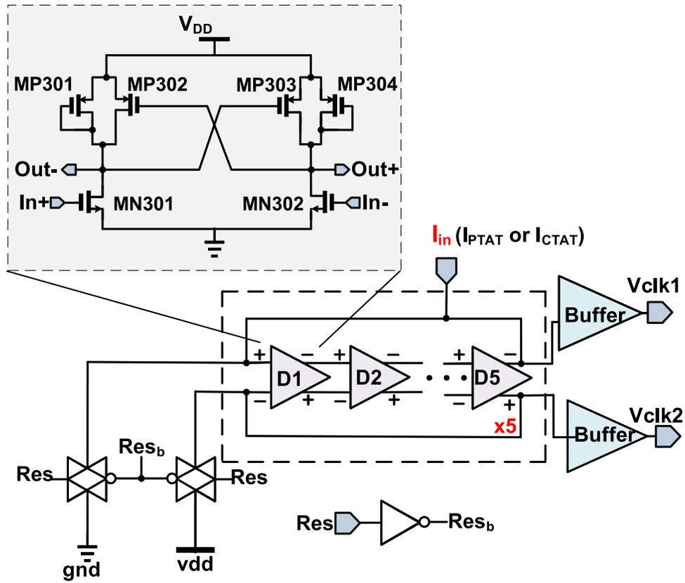
Fig. 3. Current-to-frequency converter (CFC).
