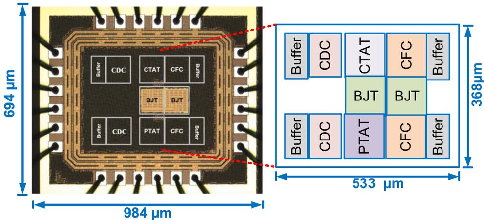
Fig. 4. Proposed temperature sensor die photo.
