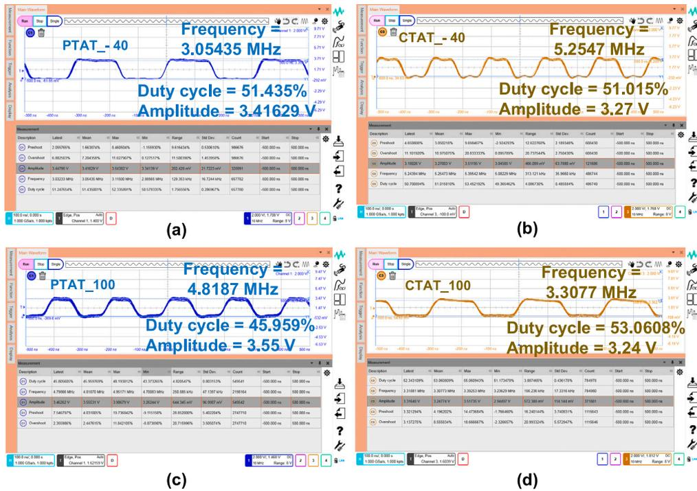
Fig. 6. The temperature to frequency measurement waveforms at (a) PTAT\_40 °C; (b) CTAT\_40 °C; (c) PTAT\_100 °C; (d) CTAT\_100 °C.
