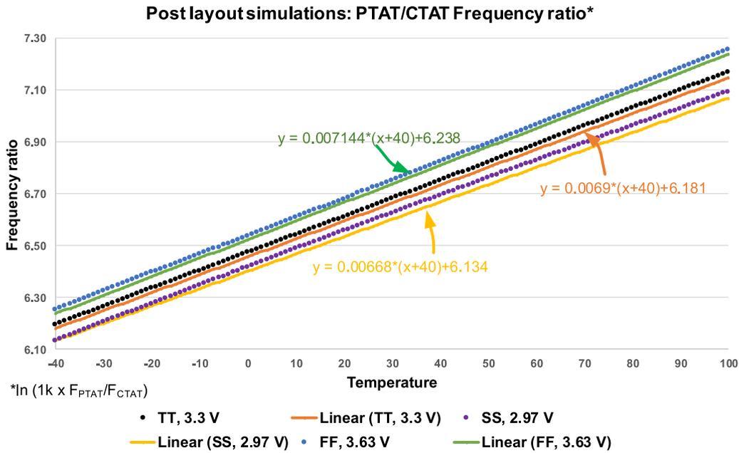
Fig. 9. The PTAT/CTAT frequency ratio curves by post-layout simulations.
