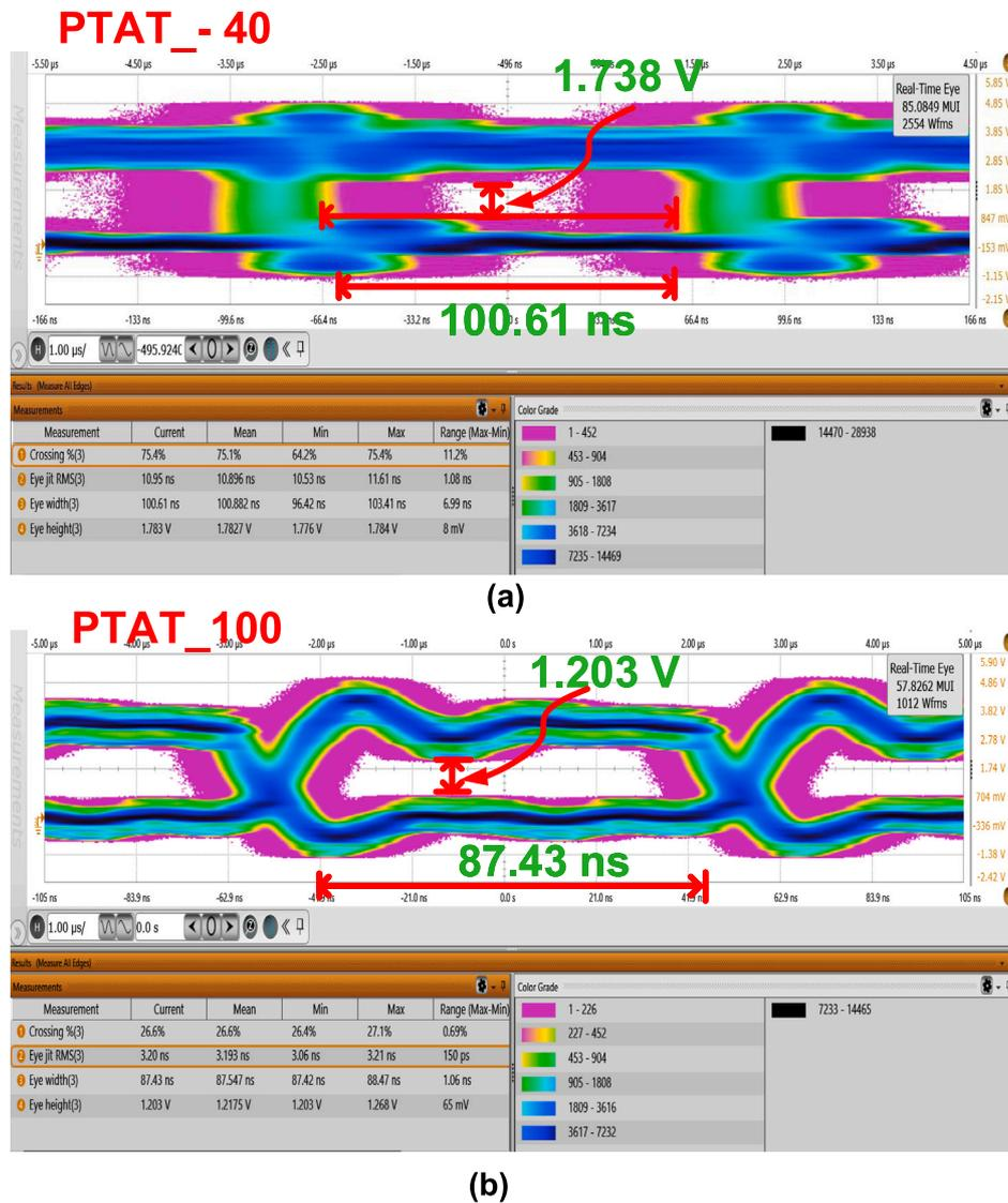
Fig. 13. PTAT Eye diagram of our temperature sensor at (a)  $-40\text{ }^{\circ}\text{C}$  and ; (b)  $100\text{ }^{\circ}\text{C}$ .
